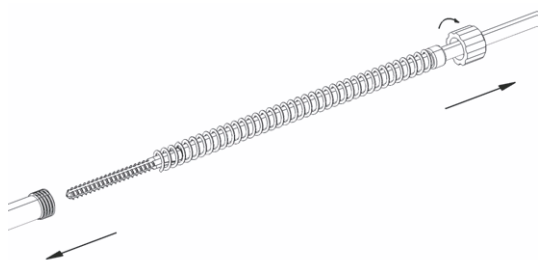
Fig. 9 Disassembling of taps
